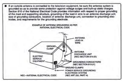
For added protection for this television equipment during a lightning storm, or when it is left unaftended and unused for long periods of time, unplug it from the wall outlet and disconnect the antenna. This will prevent damage to the equipment due to lightning and power-line surges.
